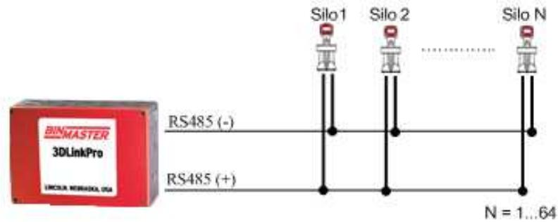
**!** Note (2): There should be a termination resistor of 120ohms between the RS485 lines; hence, placed between the positive (+) and negative (-) lines of the RS485.
