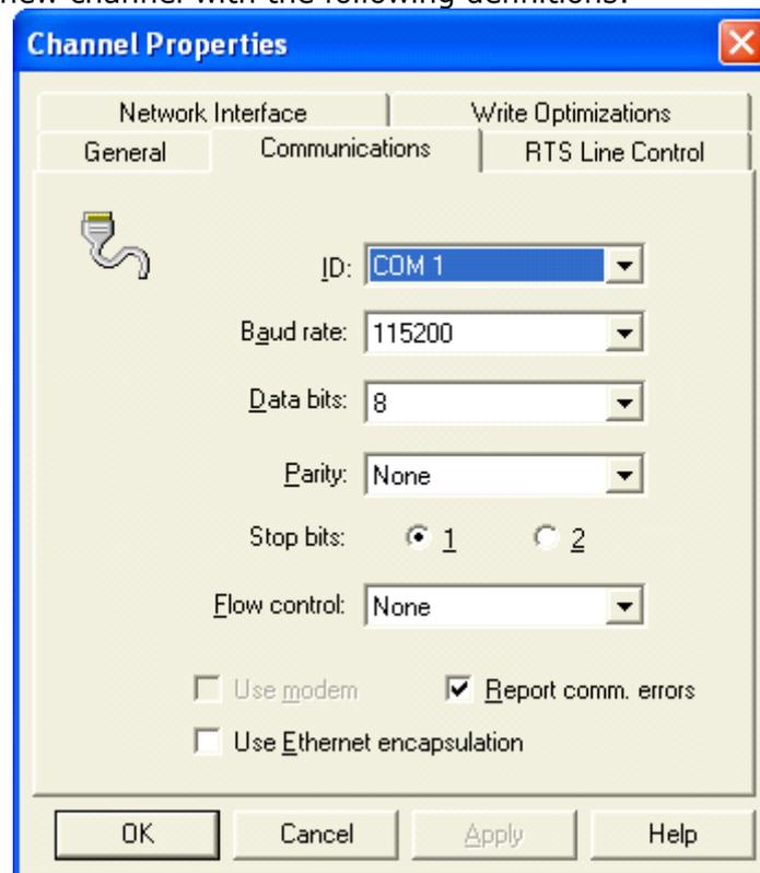
3. Add a new device (MODBUS serial) and set the following properties:
