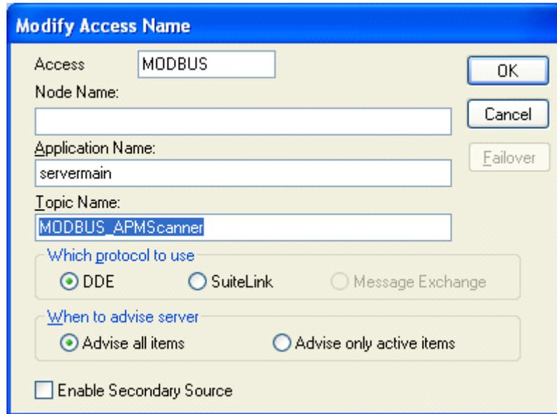
2. Topic name should be the same as the alias name in TOP Server (in this example connecting to *BinMasterScanner* device in MODBUS channel, this means the access name should be *MODBUS\_APMScanner*) see image below:
